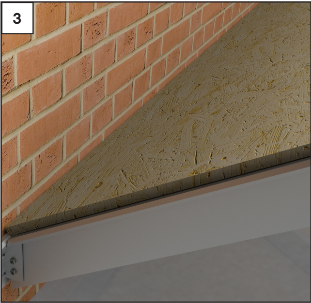
Identify and fit base panels into position. Ensure the top edge of the base panel sits against the host wall and the internal timber against the edge of the wall plate.
