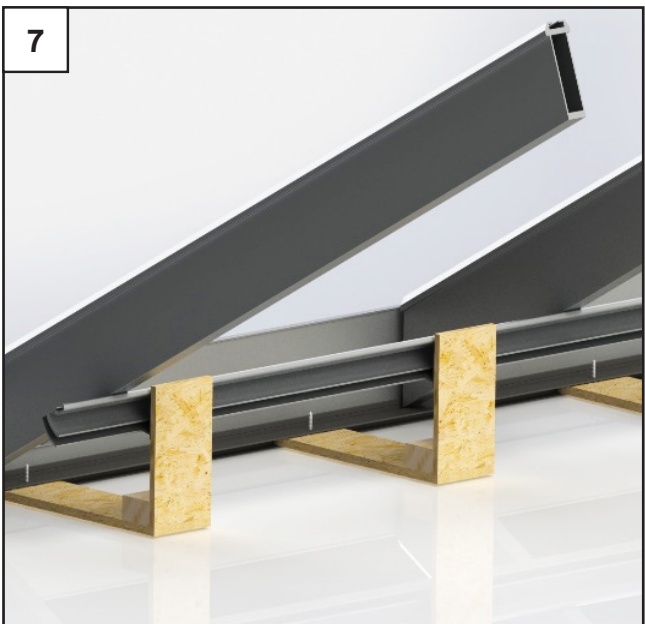
Continue to install brackets around the roof at 450-500mm centres. If roof pitches are unequal, make sure the correct width brackets go on the correct face of the roof to ensure pelmet remains a constant height around the room.
