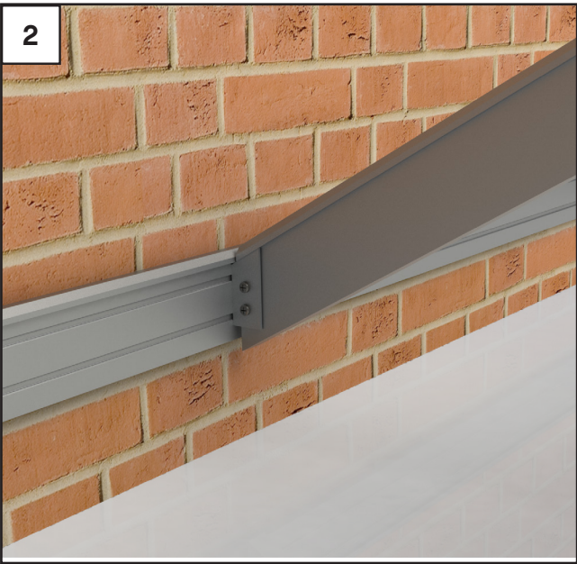
From information provided, identify and locate the rafters. Using M6x16mm Taptite screws, fix the rafters as per standard detail over the uchannel brackets on the wall plate.
