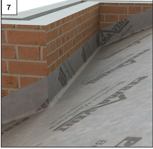
Flash roof and house wall with membrane where the flashing tray is to be installed. Take care where membrane runs up the wall into or around a corner. Note: Ensure membrane always has a min. 150mm overlap
