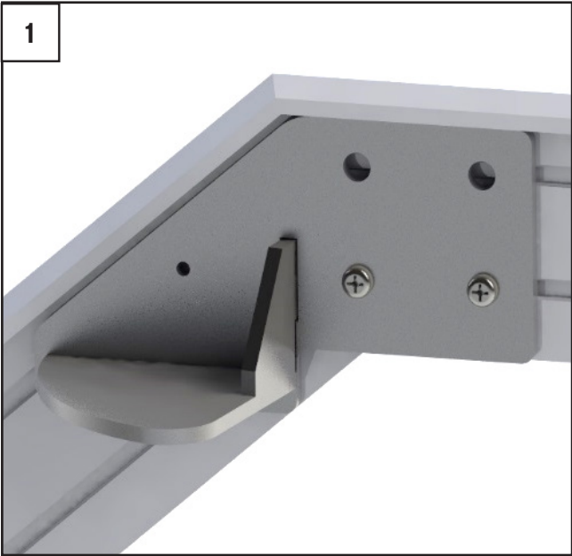
Position starter bar up to mitred edge of wall plate. Wall plate radius end should already be fixed to the wall plate. This can be done prior to fitting against wall.
