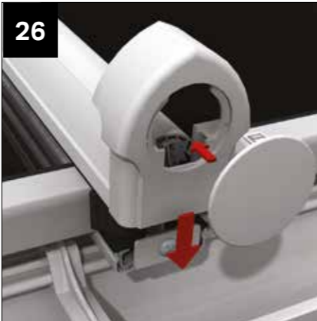
26 Fit the glazing bar end caps by sliding onto the fixing blocks. Push fit the insert into the end cap.
