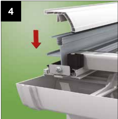
Knock the glazing bar top cappings on with a Deadblow hammer. Work your way across the roof. Once again each capping is numbered according to its position in the roof.
