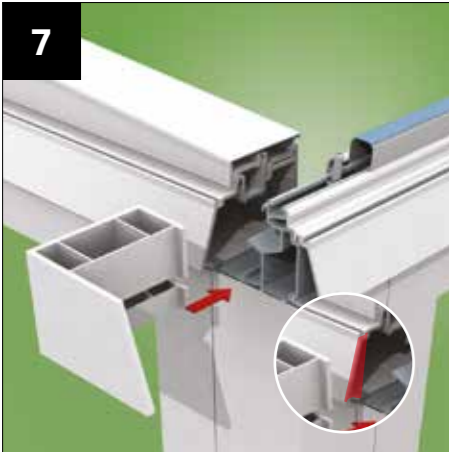
'Butter' with silicone then slide the eaves beam end cap block into place. It will be necessary to silicone seal the area highlighted in the inset image.
