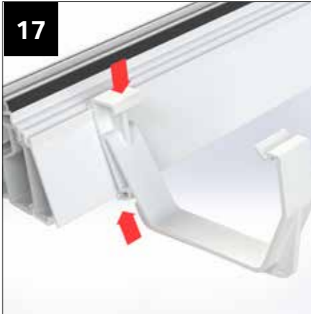
Locate the gutter bracket onto the external fascia and push down to locate the lower leg of the bracket. Assembly the outlets to the gutter profile ready for fitting. Ensure when fitting unions that the gutter is squeezed together to prevent dislodging the gasket.
