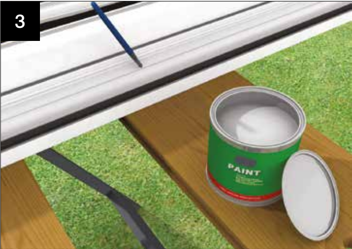
Finally, apply an air drying top coat with a fine brush.
